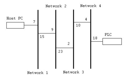
The host PC's address from the PLC's perspective is 4.2.9.7.1. The PLC's address from the host PC's perspective is 15.23.10.18.0. This is the device ID path. If the same registers were transferred from the PLC to the same locations in the host PC, the control block and data area would be used in the MSTR instruction according to the tables below. The message would be processed the same.
