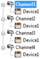
Each device can be defined under its own channel. In this configuration, the server can dedicate a single path of execution to the task of gathering data from a single device because each has its own dedicated channel. If the application has fewer devices it can be optimized as displayed.
