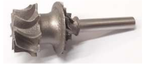
Cantilevered Inconel Monolithic Rotor Operated at Design Speed of 500 kRPM
