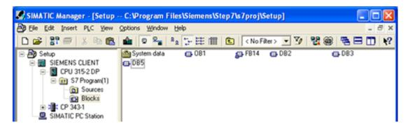
2. Double-click on **DB5**, then specify a memory size. Although the array size in this example was chosen arbitrarily, the values should be specified to fit a particular need.
