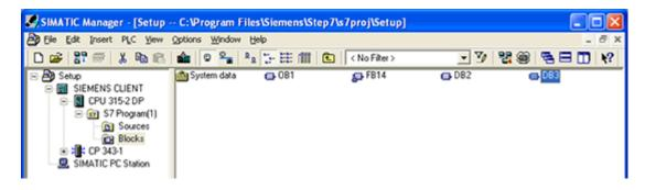
3. Double-click on **DB3**. To assign some memory to the data block, users can make changes similar to those shown below. Although the array size in this example is arbitrary, values should be specified to fit a particular need.
