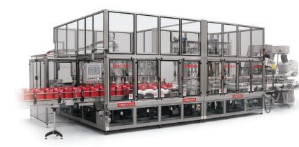
and built for the customer. This equipment also has a very long lifespan, and it evolves over time to process new bottles and caps formats through mechanical/software modifications.
