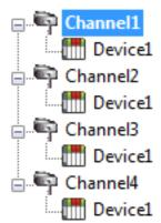
Each device has now been defined under its own channel. In this configuration, a single path of execution is dedicated to the task of gathering data from each device. If the application has 1024 or fewer devices, it can be optimized exactly how it is shown here.
