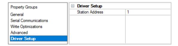
**Station Address**: This driver only issues requests when it's polled by the Uni-Telway network controller. The assigned station address determines which poll request the driver responds to in the programmed sequence. Valid range is from 1-253.
