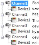
Each device can be defined under its own channel. In this configuration, a single path of Device1 execution is dedicated to the task of gathering data from each device. If the application has fewer devices, it can be optimized exactly as shown here.
