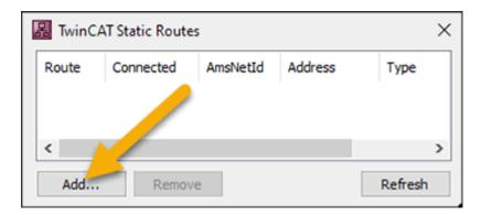
5. Enter the host name or IP address of the remote system (or perform a broadcast search for TwinCat PLCs and select the PLC from the list).
