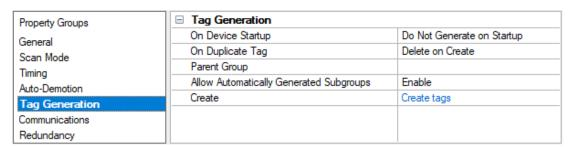
**On Property Change**: If the device supports automatic tag generation when certain properties change, the **On Property Change** option is shown. It is set to **Yes** by default, but it can be set to **No** to control over when tag generation is performed. In this case, the **Create tags** action must be manually invoked to perform tag generation.
