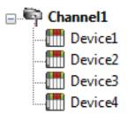
Channel1 In this example, each device appears under a single channel. In this configuration, the driver must move from one device to the next as quickly as possible to gather information at an effective rate. As more devices are added or more information is requested from a single device, however, the overall update rate begins to suffer.
