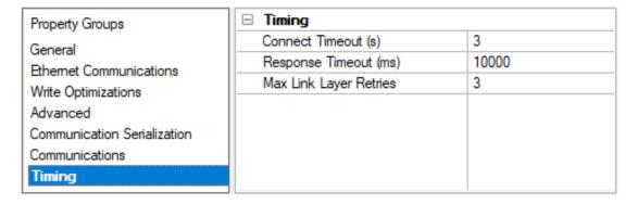
**Connect Timeout (s)** This property specifies how long the device waits for a connection request to complete before timing out. The valid range is 1 to 30 seconds. The default setting is 3 seconds.
