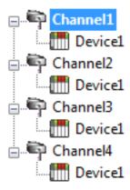
Each device can be defined under its own channel. In this configuration, a single path of execution is dedicated to the task of gathering data from each device. If the application has 100 or fewer devices, it can be optimized exactly how it is shown here.
