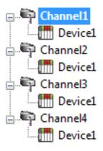
Each device can be defined under its own channel. In this configuration, a single path of execution is dedicated to the task of gathering data from each device. If the application has fewer devices, it can be optimized exactly how it is shown here.
