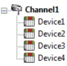
Each device appears under a single channel. In this configuration, the driver must move from one device to the next as quickly as possible to gather information at an effective rate. As more devices are added or more information is requested from a single device, the overall update rate begins to suffer.
