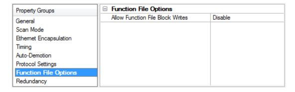
For applicable function files, data can be written to the device in a single operation. By default, when data is written to a function file sub element (field within the function file structure), a write operation occurs
