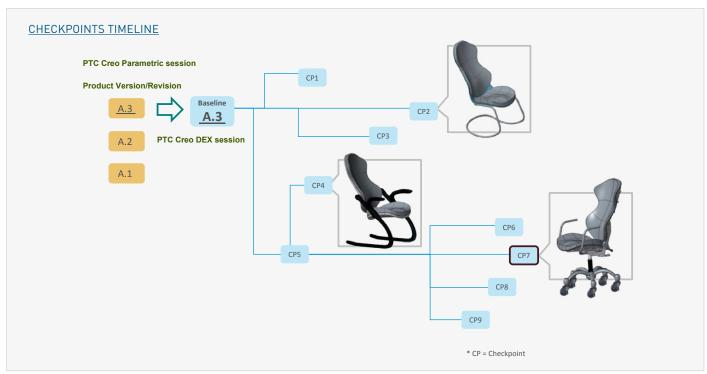
PTC Creo DEX allows users to switch back and forth between stored checkpoints enabling exploration and evaluation of different design ideas.
