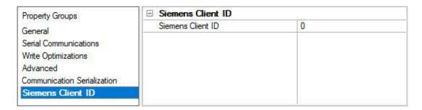
**Siemens Client ID**: Specify the node number used by the Siemens S7-200 Driver on the network. Each channel must have a unique Siemens client ID. The valid range is 0 to 126.
