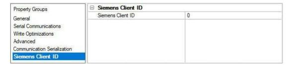
**Siemens Client ID**: Specify the node number used by the Siemens S7-200 Driver on the network. Each channel must have a unique Siemens client ID. The valid range is 0 to 126.
