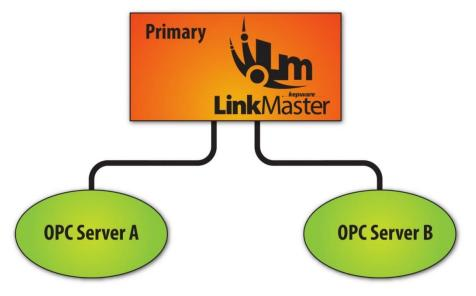
LinkMaster can also be used as a data concentrator by connecting to multiple OPC servers and providing a single OPC server interface to other OPC Clients.
